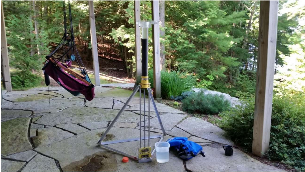
Figure 6: South Bay west sediment core in extruder ready for sectioning in the field.
