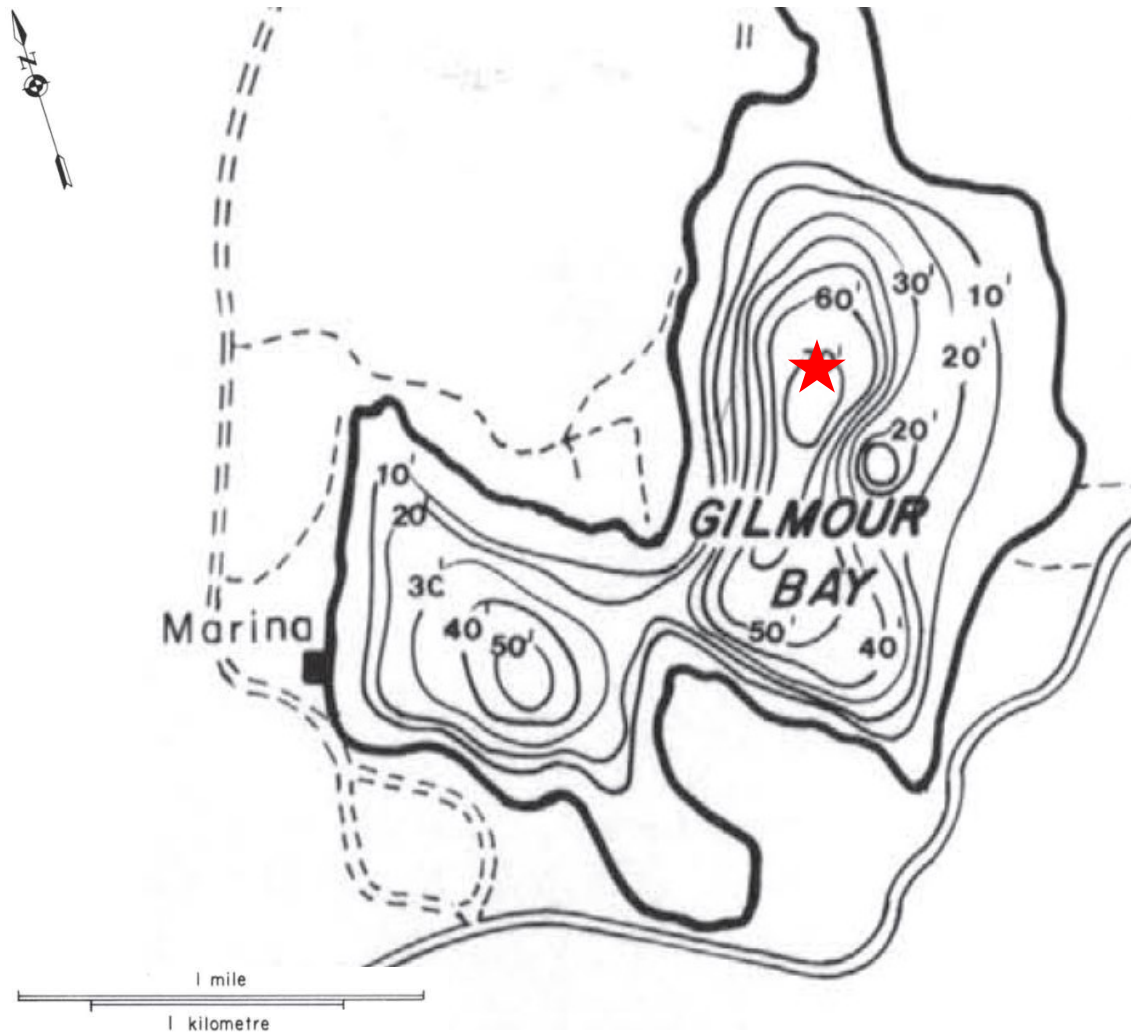
Figure 3: The bathymetry of Gilmour Bay including the coring location (red star). Contour lines represent 10 ft intervals beginning at 0 ft along the shoreline. Revised from The Angler's Atlas (2007).
