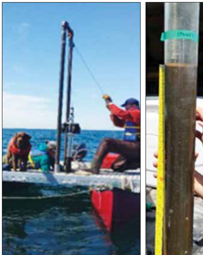
Fig. 3. Coring platform used in this project. The platform is mounted across two structurally-reinforced canoes. The Glew gravity corer was equipped with an 80-cm core tube, and weighs approximately 28 kg. The chocolate Lab Sasha is wearing a Ruffwear life jacket. The sediment core from Stony Lake is shown on the right.
